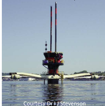
SeaGen 1.2MW tidal turbine produced by Marine Current Turbines Ltd. - rotors in 'raised for maintenance' position.
