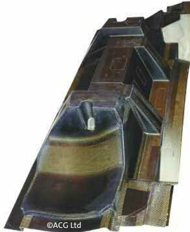
ACG DForm tool, created from the master model, used to manufacture the bulkhead for the E-4 Coupé.
